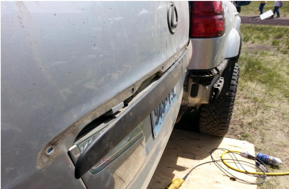
After removing this trim piece, you'll gain access to two small bolts holding the backup camera into place. Remove these bolts.
