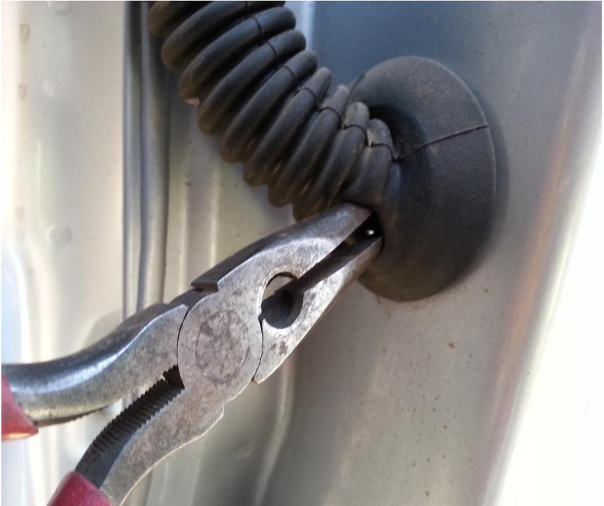
Mark the length of harness you'll need to run the wires through the factory door grommet and to the 4 OEM wires you just cut. Use the heat shrink around the supplied wire harness. Leave approximately 8-10 inches of wire and plug hanging out of the door grommet.
