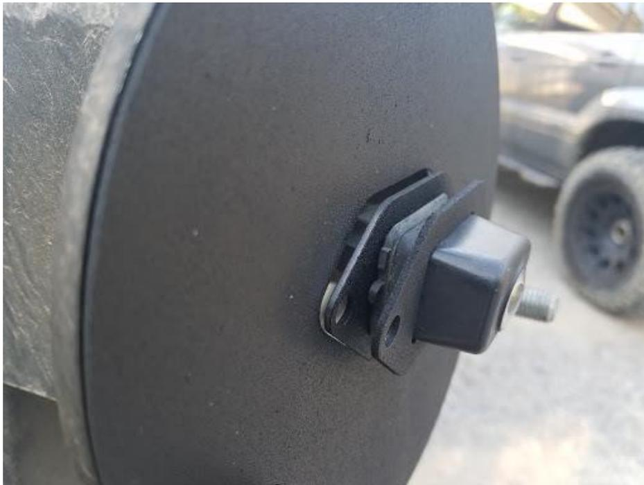
Tighten the provided ¼" button head bolts and nuts so that the camera is snug.
