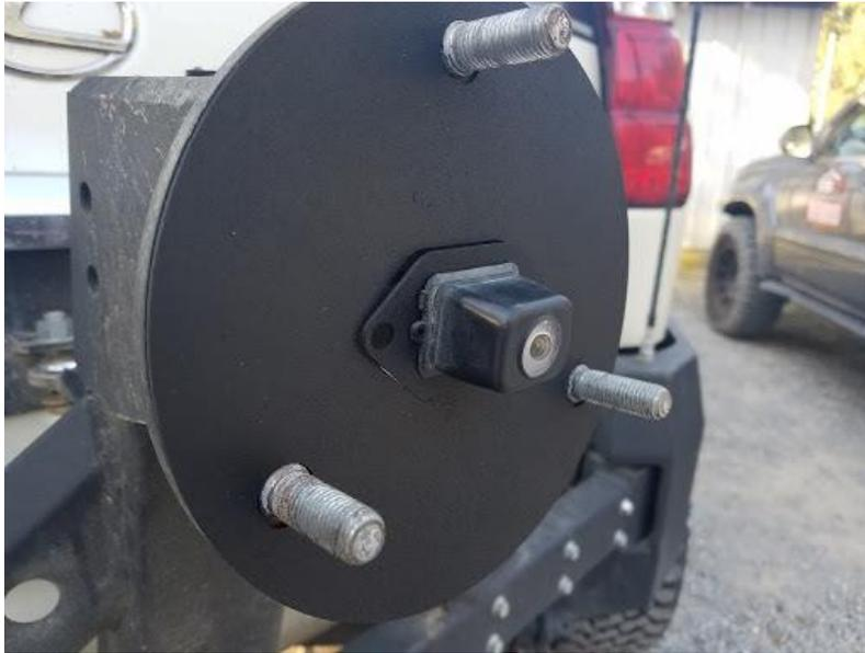
Sandwich the camera between the back plate and the adapter plate
