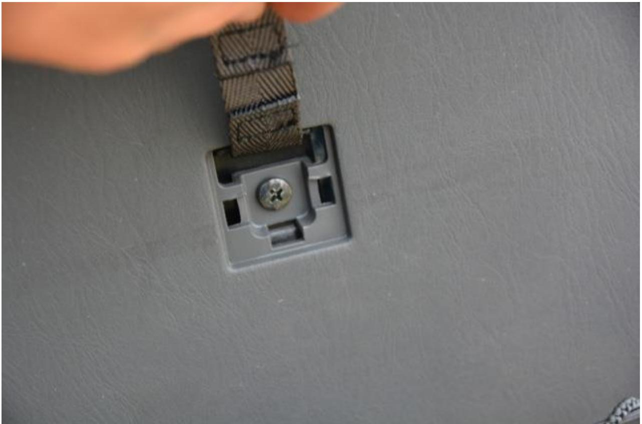
Using a panel removal tool or flat head screwdriver, carefully pry up the bottom corner of the back door panel. You'll be able to hear and feel each plastic pin pulling out as you move around the edge of the door.
