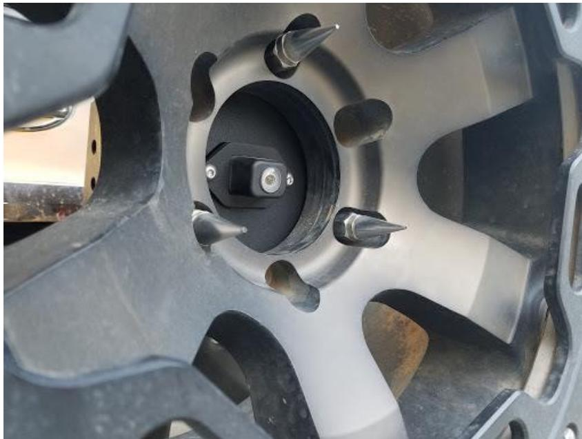
Verify that the picture is clear. You can adjust the angle of the camera at any time, however it was not designed for constant adjustment. The metal may fatigue and snap if adjusted up and down too many times.
