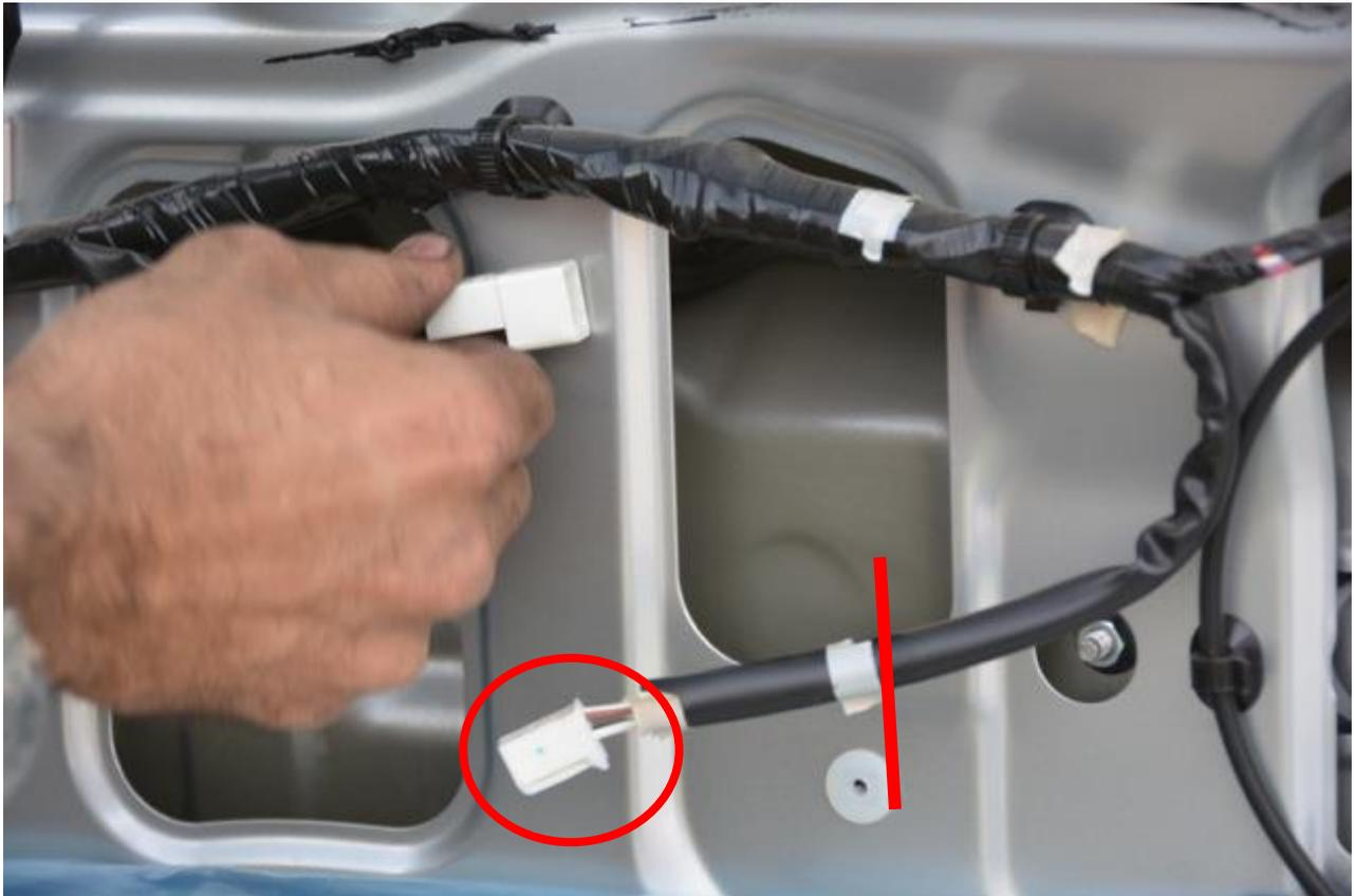
Cut the OEM wiring harness at the point indicated in the picture above. **It is important that you make this cut so that there are 4 wires and not 3.** One of those wires is a shielded cable that splits off into 2 near the electrical connector.
