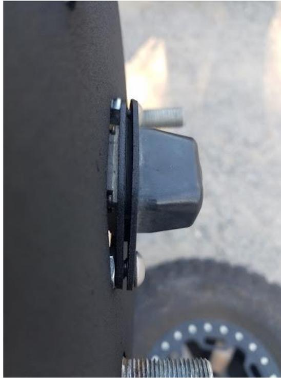
You'll also notice that the camera back plate has been cut so that you can easily bend the camera into the position that best suits your install. This will help keep the camera focused directly behind you instead of off into the distance.
