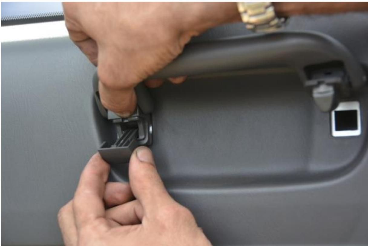
After removing plastic pins on both side of the handle, pull down and away to remove handle from frame of door
