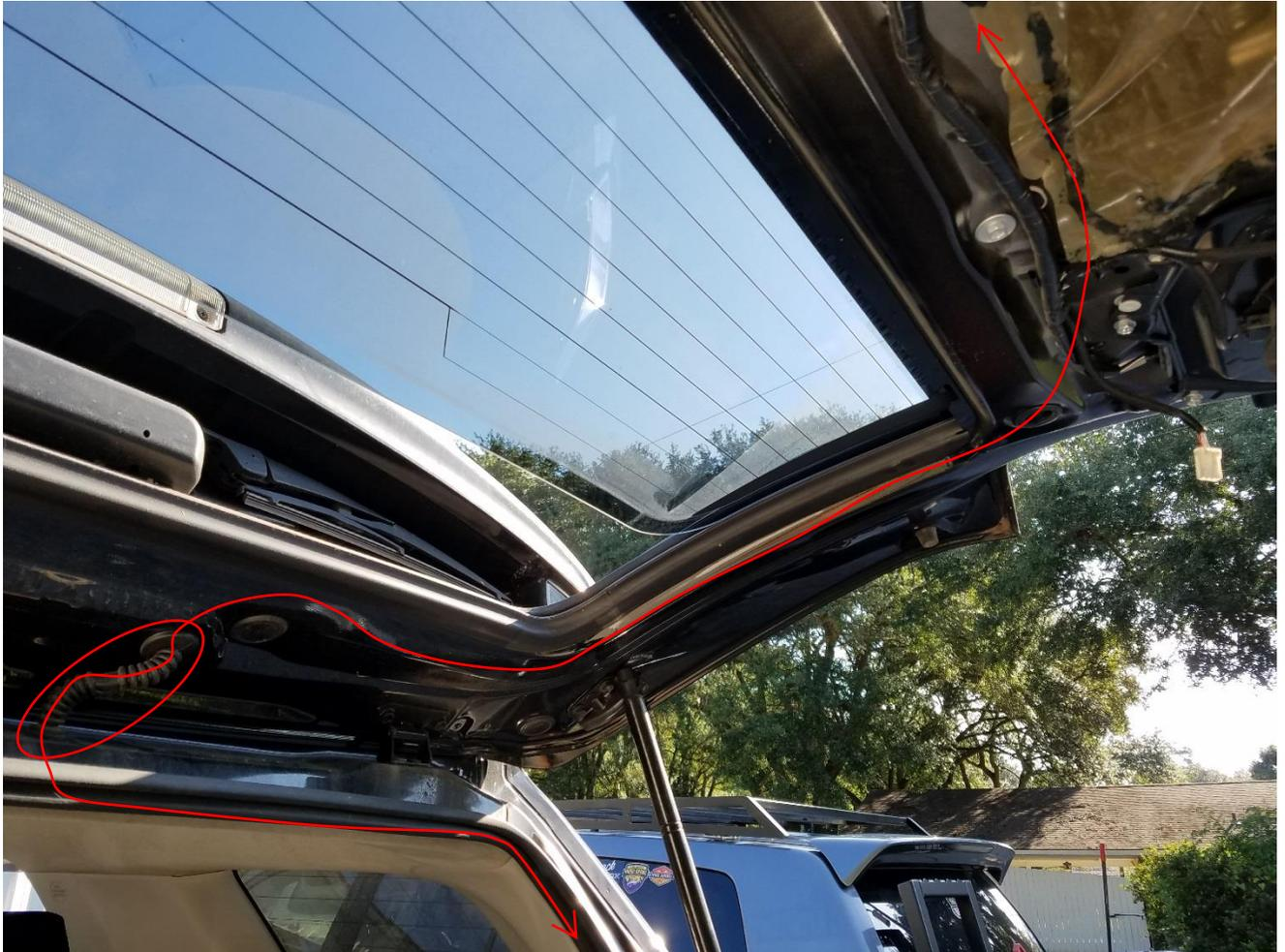
Use the heat shrink around the supplied wire harness. Leave approximately 8-10 inches of wire and plug hanging out of the passenger taillight area.
