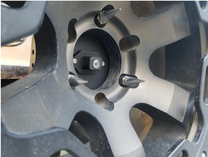
You'll also notice that the camera back plate has been cut so that you can easily bend the camera into the position that best suits your install. This will help keep the camera focused directly downward and behind you instead of off into the distance. Verify that the picture is clear. You can adjust the angle of the camera at any time, however it was not designed for constant adjustment. The metal may
