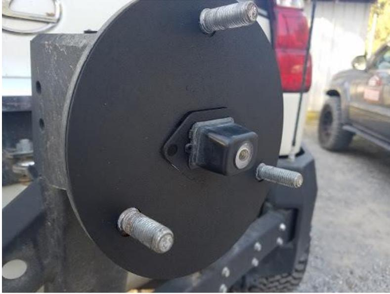
Using the supplied 1/4" button head bolts and nuts fasten the adapter plate to the back plate. Install your rear tire.
