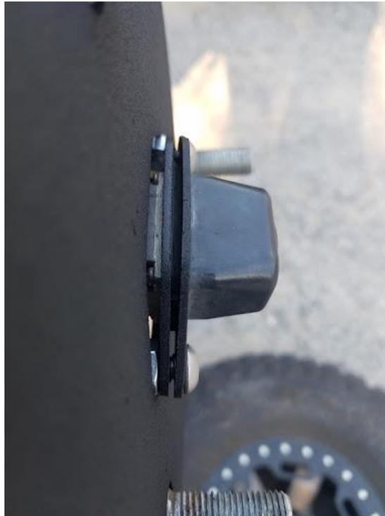
After you've successfully run the wires and tested the camera, you can install the camera onto your tire carrier. Begin by placing the back plate onto your tire carrier and feed the camera and plug through the large hole in the center of the back plate.
